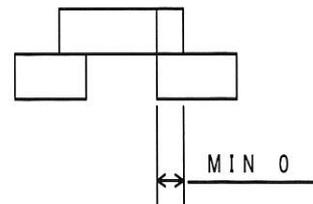
Component position (A) on solder pad should be less than 1/2 width of IC lead..
